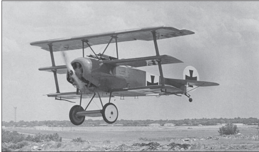
Figure 4.64 The World War I Fokker Dr-1 triplane, the first fighter aircraft to use a thick airfoil. (© Ed Maker/The Denver Post via Getty Images).
