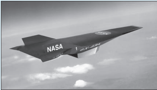
(b) SCRAMjet-powered X-43 experimental air breathing hypersonic vehicle.
