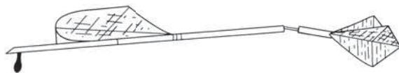
Figure 4.59 The first modern configuration airplane in history: George Cayley's model glider of 1804.
