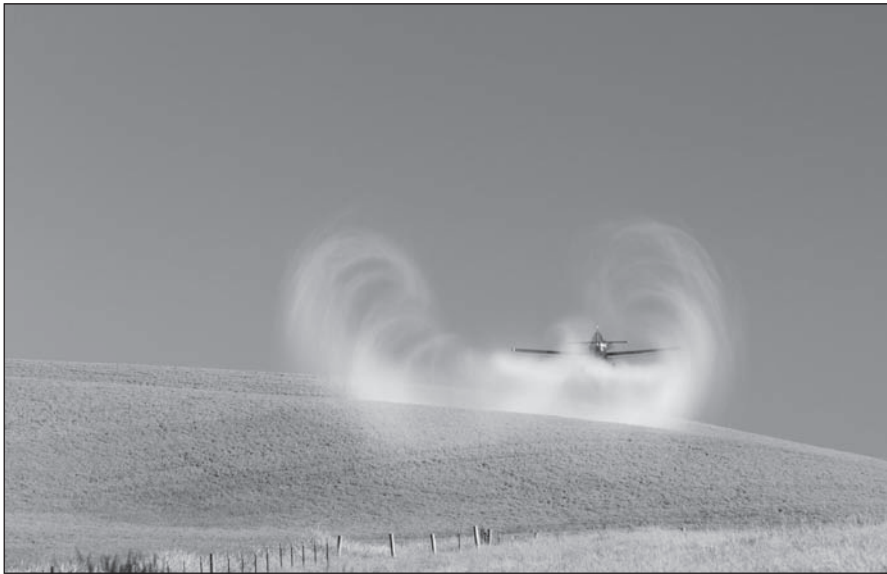
Figure 5.5 Wing-tip vortices from a finite wing. (© Steve Whiston – Fallen Log Photography/Getty Images ).
