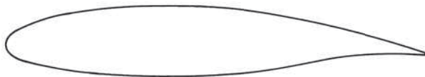
Figure 4.36 Profile for the NASA LS(1)-0417 airfoil. When first introduced, this airfoil was labeled the GA(W)-1 airfoil, a nomenclature which has now been superseded. (From McGhee, R. J., and W. D. Beasley: Low-Speed Aerodynamic Characteristics of a 17-Percent-Thick Airfoil Section Designed for General Aviation Applications , NASA TN D-7428, December 1973.)
